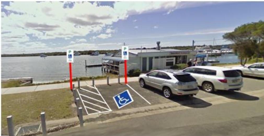
Signs and Pavement markings to designate Disabled Parking Space and Shared Area access
