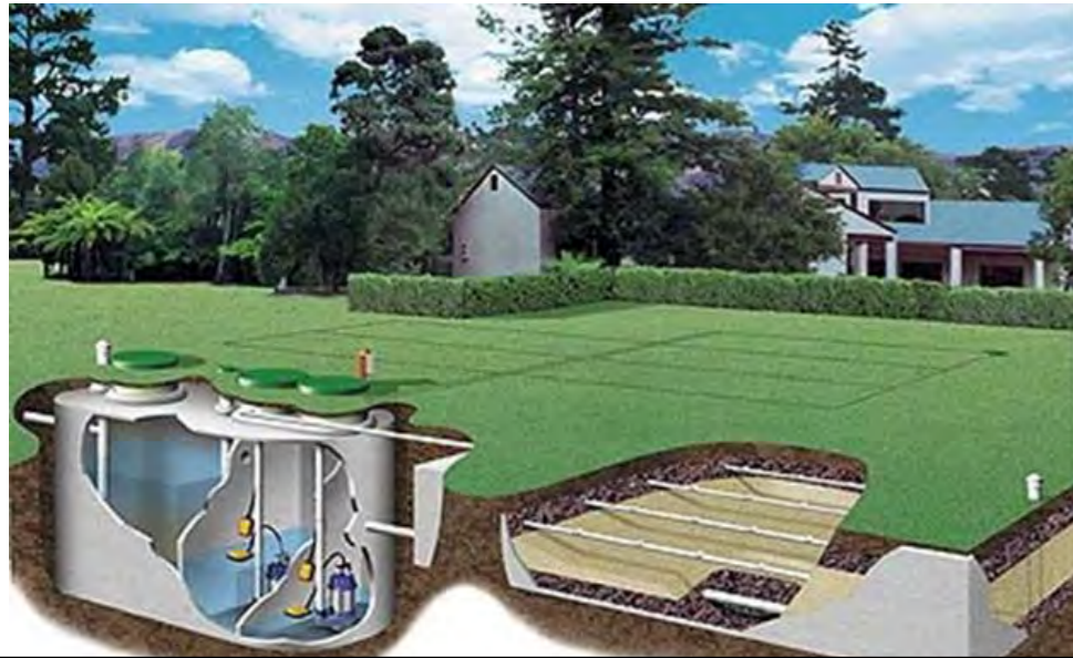
Recirculating sand filter with subsurface irrigation
