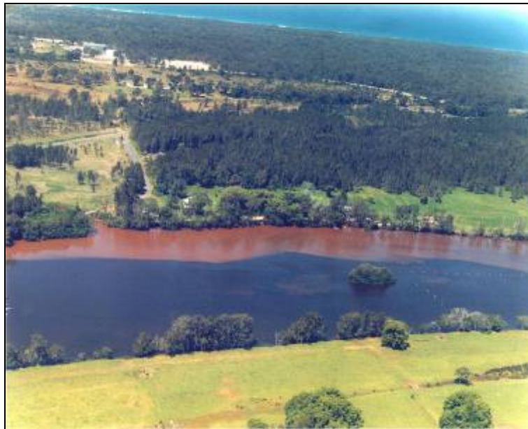
Figure 20: An acid sulphate plume entering the Wallamba River from Darawank Creek.
