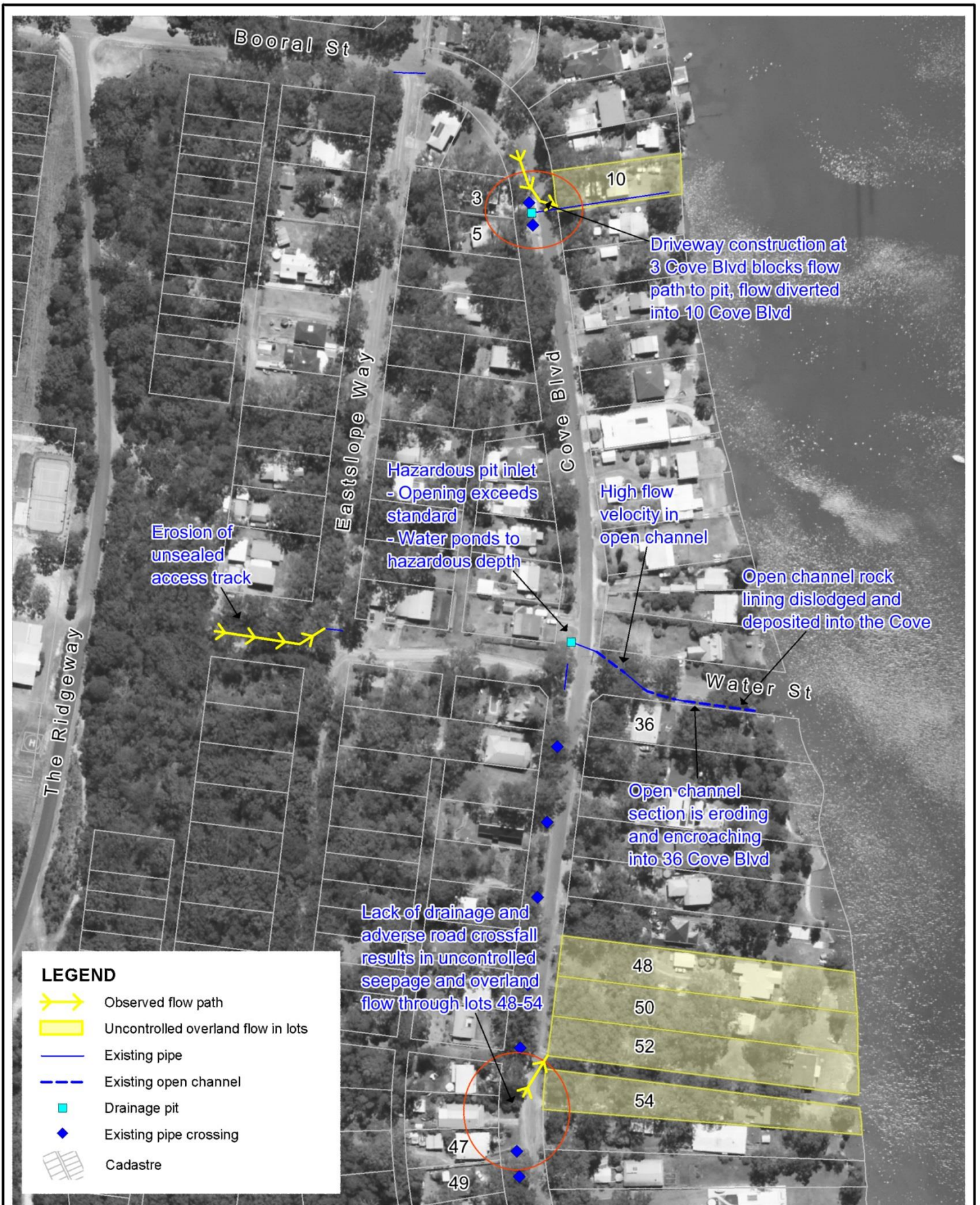
Title: Sites 2a, 2b and 2c - Existing Stormwater Management Issues
