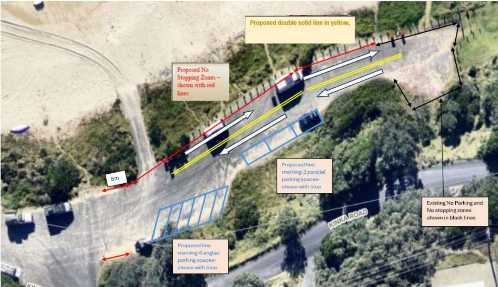
ATTACHMENT E: Map showing proposed double solid line and No Stopping signage at Kinka Road adjacent to Boat Beach.
