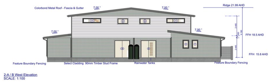
Figure 8: 2A & 2B Western Elevation (Source – RaP Drawing)
