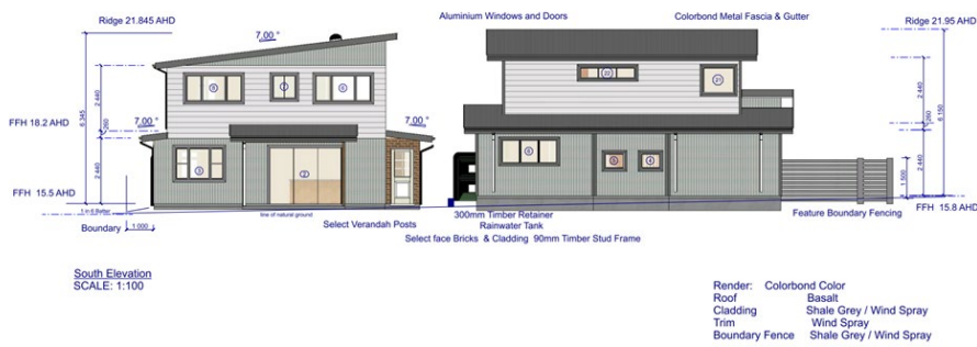
Figure 7: Southern Elevation (Source – RaP Drawing)
