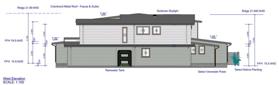
Figure 9: 2C Western Elevation (Source – RaP Drawing)
