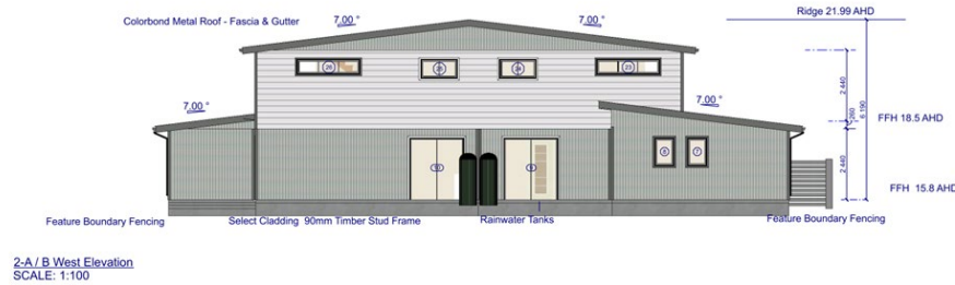
Figure 8: 2A & 2B Western Elevation (Source – RaP Drawing)
