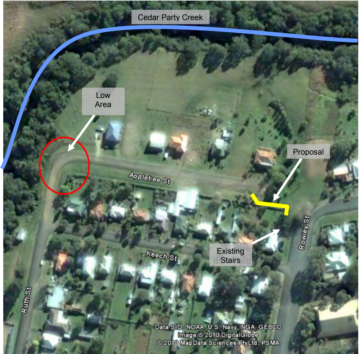
Figure 9: Location of the proposed footway connecting West Appletree Street with Rowley Street in order to bypass the low area.
