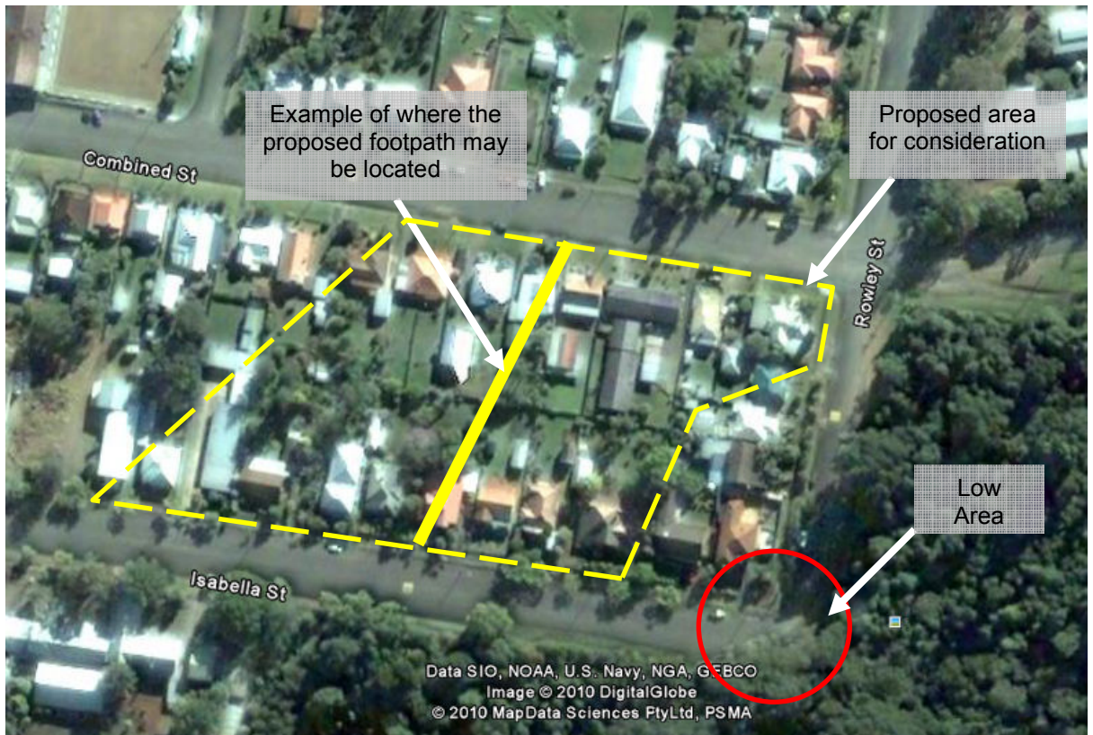
Figure 10: Location of the proposed footway connecting the high ground on Combined and Isabella Streets in order to bypass the low area at the intersection of Rowley and Isabella Streets.
