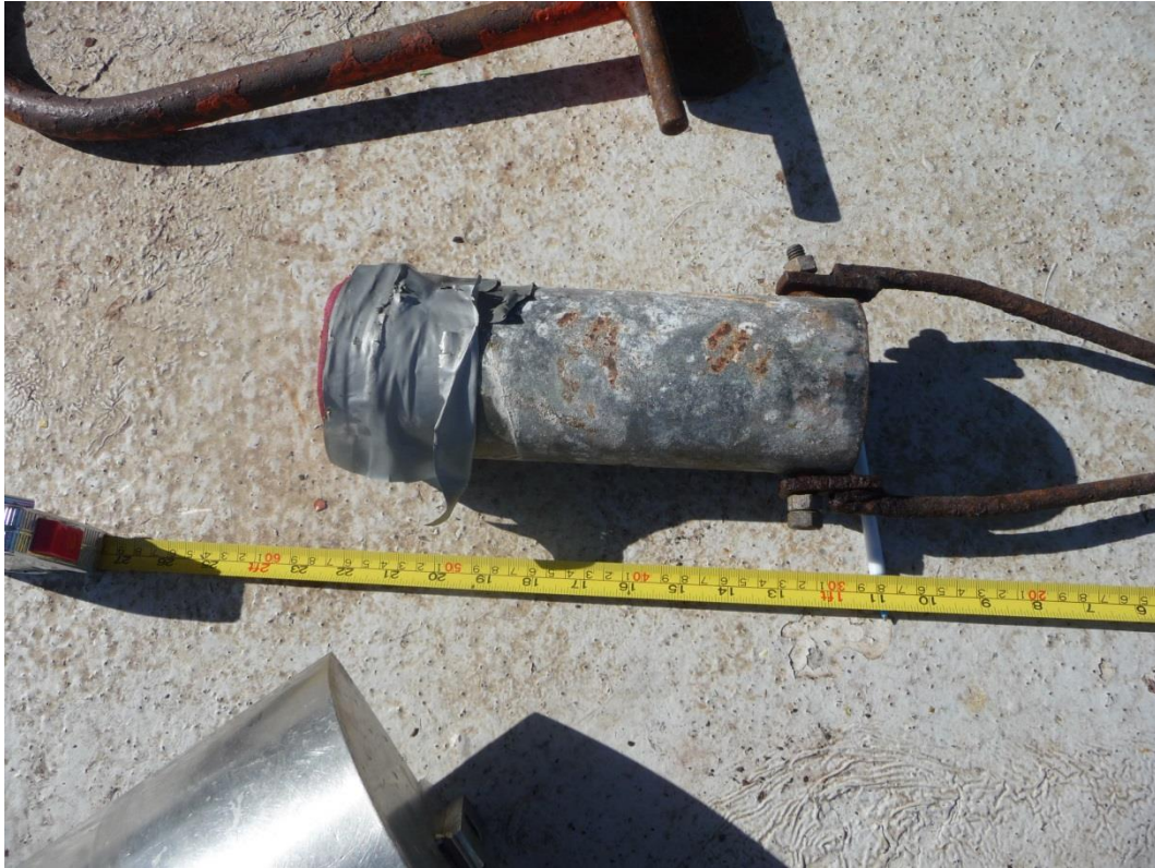
Figure 23: Dredge pipe used for surf-zone sampling, 9 July 2014
