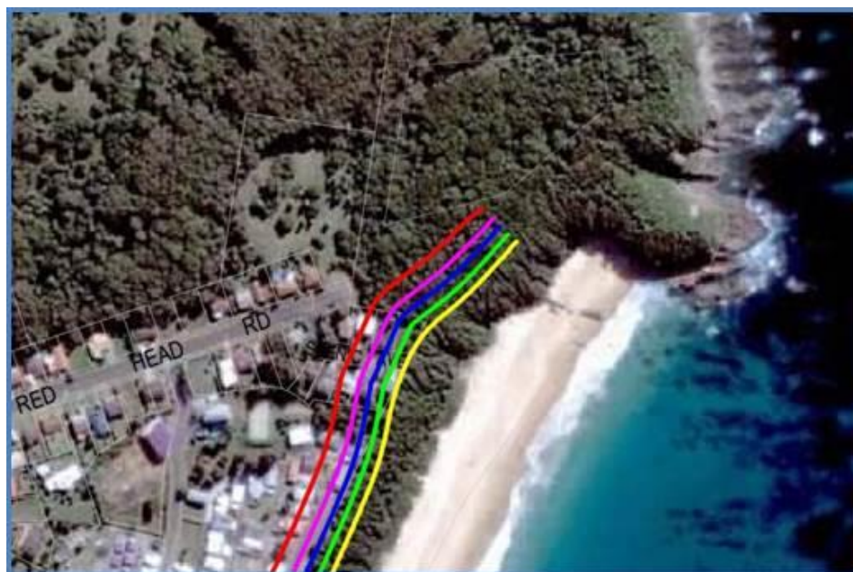
Figure 2: Red Head Hazard Lines (Worley Parsons, 2010)
