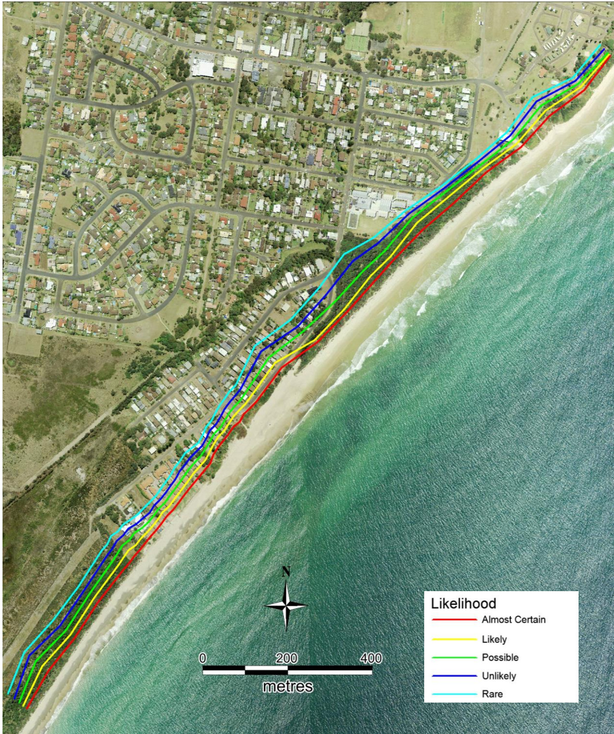
Figure 8: Likelihood lines at Old Bar Beach for Type 1 procedure (no recession included)
