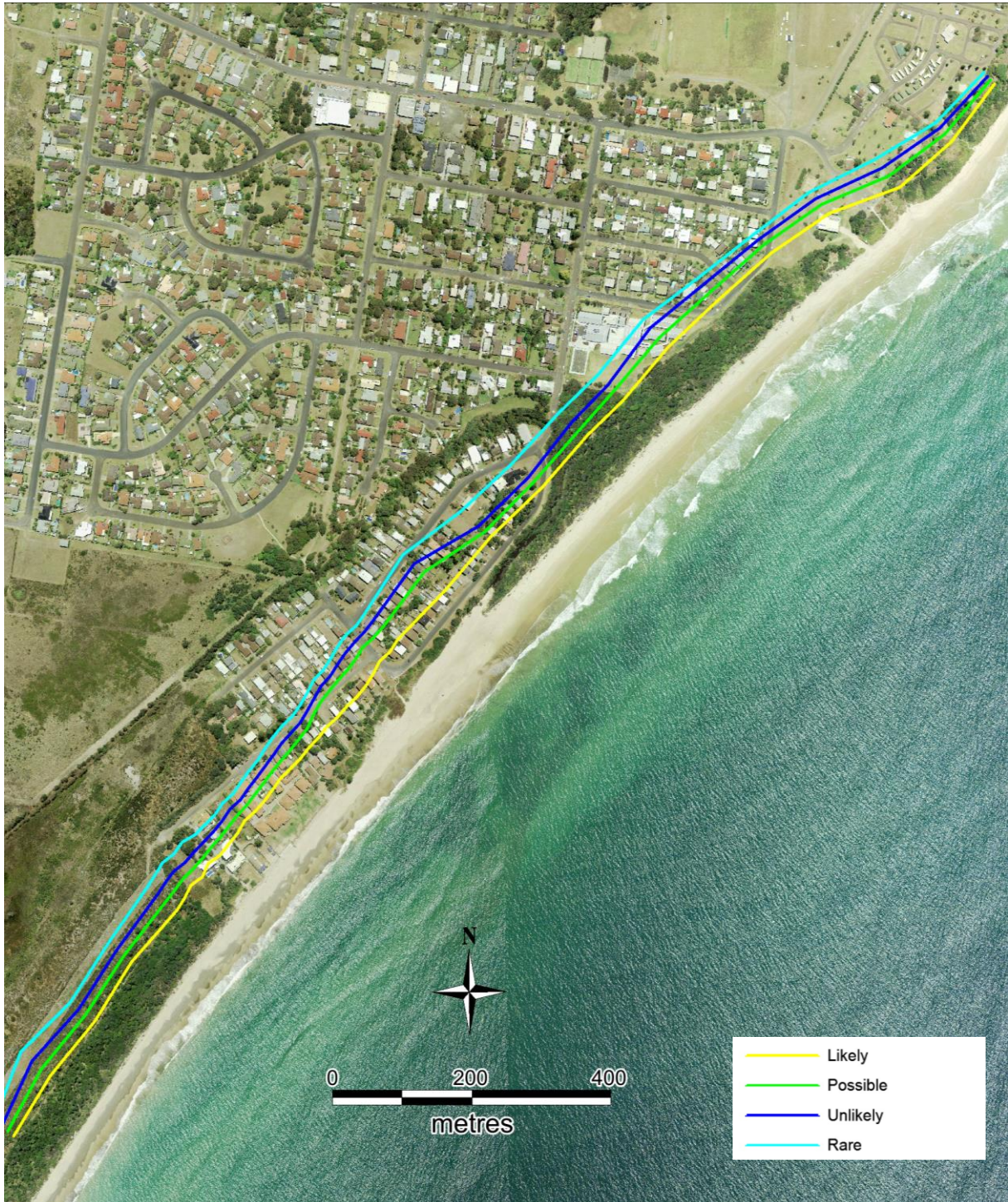
Figure 10: 50% exceedance recession scenario likelihood lines at Old Bar Beach for Type 2 procedure
