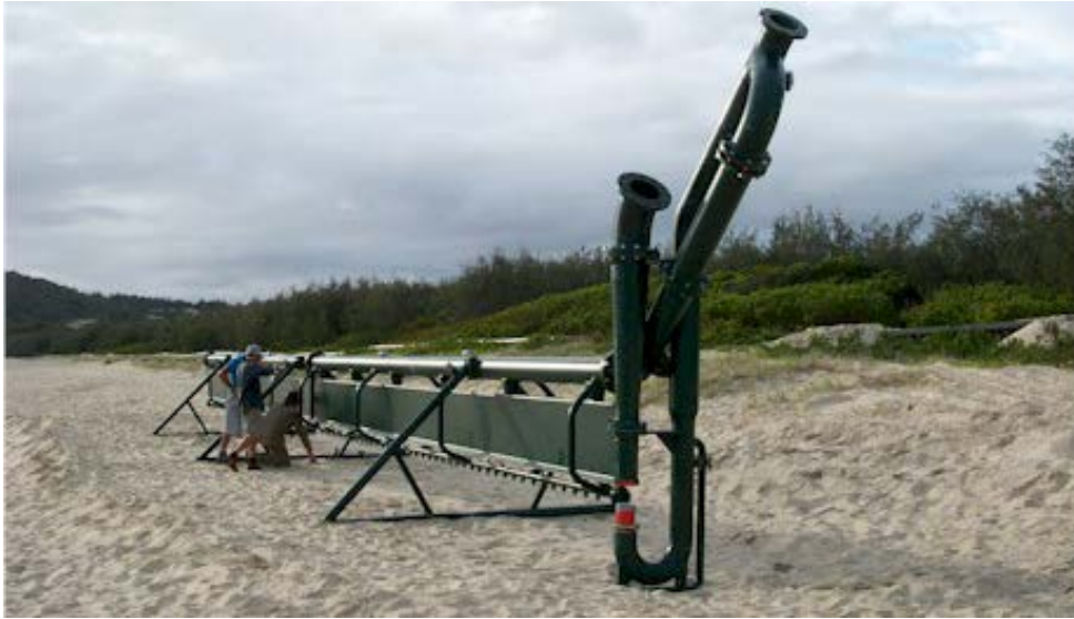
Figure 4 Typical Sand Shifter Unit Configuration (source: Slurry Systems Marine)
