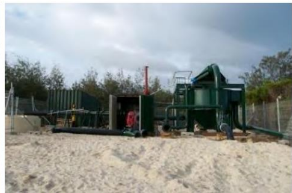
Figure 5 The Noosa trial Sand Shifter unit sourcing sand from the shore (left) and onshore booster pumps and pipework (right)
